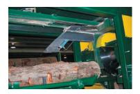
The Pendu Model 6800 Scragg Mill takes raw logs and turns them into workable cants quickly and efficiently.
